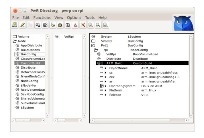
Open the root volume, in the example VolRpi, execute the basic configuration with the wizard, and then open volume attributes from File/Volume Attributes in the menu. Set OperatingSystem to *CustomBuild*.
